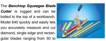
100 durometer. Made from gold anodized aluminum, the unit comes with a set of five replacement blades, a scale and a fine adjustment rod for setting blade lengths for repeat cuts.
