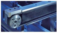
Automatic conveyor width adjustment, software control flow direction(L>R,R>L.L>L,R>R) and the highly durable Antistatic U-shape belt are all standard features, Conveyor belt is driven by stepper motor with a precision control of PCB soft stop position.
