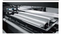
A two ways automatic wet/dry/vacuum stencil wiper allows user to select any combination of cleaning mode to best suit their application
