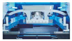
The Arch Shape Squeegee Beam is made by solily casted high intensity steel material, It proveds the rigidity and the durability to the entire squeegee assembly for stable and balance squeegee movement.
