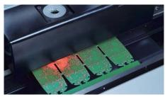
The simultaneously Look Up/Look Down optical camera system adopted uniform ring light and high brightness coaxial light, equipped with adjustable brightness control can handle allk inds of fiducial marks with high resolution and precision.
