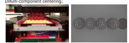
[Multi-component centering] Up to 4 components are centered in a single image. Sample images
